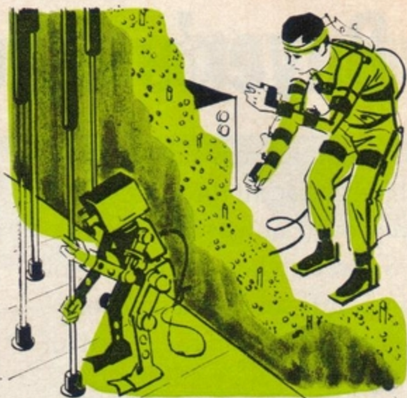
A miniature version, exposed to radioactivity, works to free jammed control rod of a nuclear reactor as operator watches on a TV monitor.
