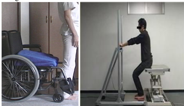
Fig. 2 active chair embedded assistant (a) Sit-to-stand motion aid for a wheelchair using the MH air compressor. (b) adaptive support system for sit-to-stand movement from a bed
