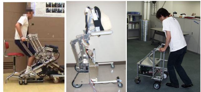
Fig. 5 (a) MONIMAD. (b) Standing assistance system (c) RT WALKER
