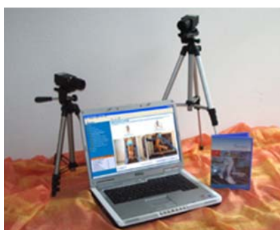
Fig. 4. CONTEMPLAS motion analysis equipment
