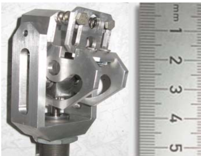
Fig. 19. Real model of parameterized knee prosthesis for children
