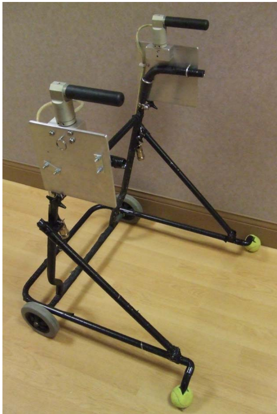
Figure 4.7. Instrumented walker with load cells to measure vertical upper extremity forces.
