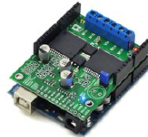
Pololu dual VN5019 motor driver shield, assembled and connected to an Arduino Uno.
