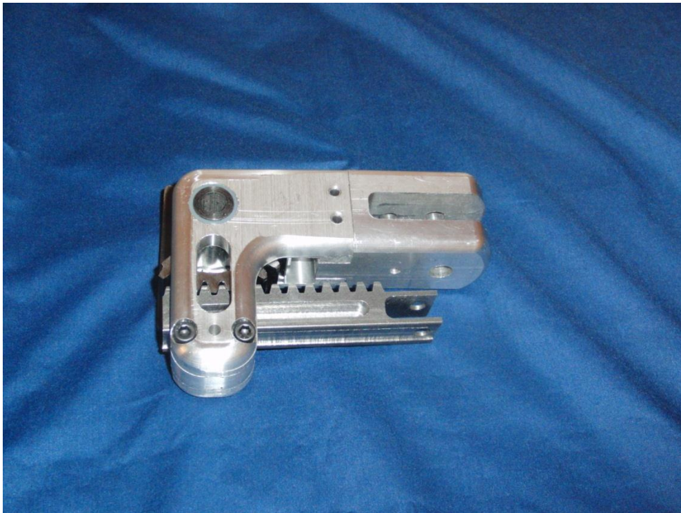
Figure 7 – A completed and assembled VCHM gear assembly.
