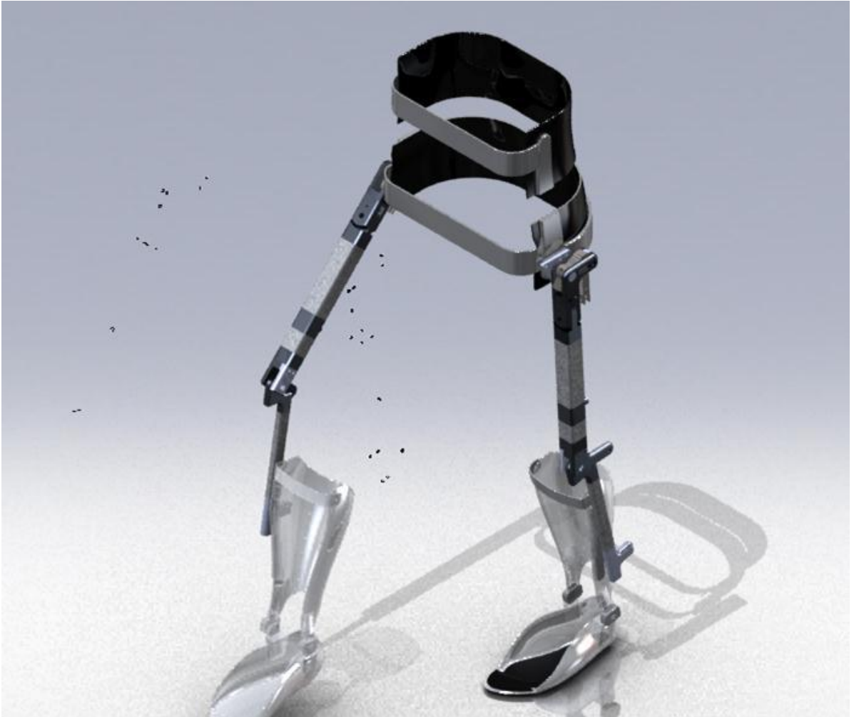
Figure 12 – CAD model of the modified HNP design.
