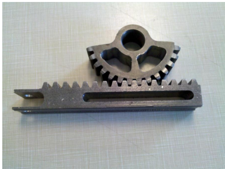
Figure 6 – A manufactured modified rack and pinion gearset.
