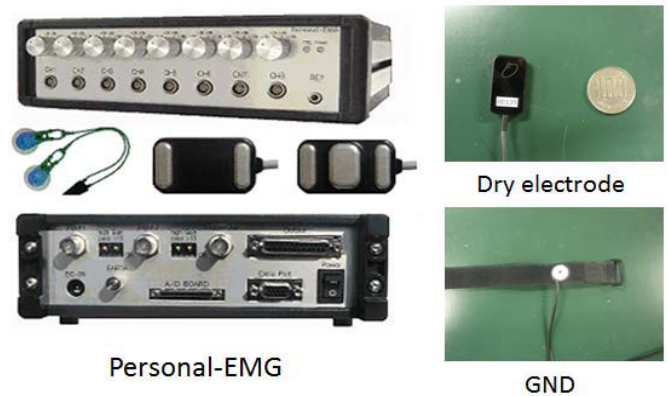
Fig. 7. Experimental setup of sEMG acquisition
