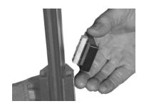
2. Insert the T-Nut into Keyed Back Post channel and position the MR-8 Mount Adapter at the marked location (see Preparing Mount Base #1). Tighten the two T-Nut screws.
