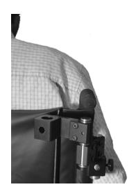
7. Snug but do not tighten the six Clamp Screws using the large T-Wrench. Add enough tension so that the joints do not move easily but can be repositioned if required to optimize the arm alignment.
