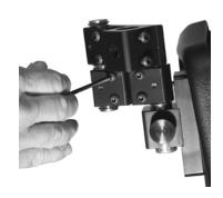
11. Hold the Pitch Mount Shaft so that the black Pitch Pivot is at the proximal end, the hole through the Pitch Pivot is in the line of progression of the chair and the plate of the pivot is facing laterally. Insert the Pitch Mount Shaft into the Mount Shaft Base. Snug but do not tighten the screws on the Mount Shaft Base.
