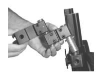
6. Preposition the Mount Links so that the Mount Shaft Base that receives the Pitch Mount Shaft is located in the lateral 1/3 of the clients torso on the side which you intend to use the WREX Arm.
