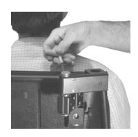
10. Snug <u>but do not tighten</u> the **six** Clamp Screws using the Large T-Wrench. Add enough tension so that the joints do not move easily but can be repositioned if required to optimize the arm alignment.
