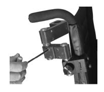
8. Hold the Pitch Mount Shaft so that the black Pitch Pivot is at the proximal end, the hole through the Pitch Pivot is in the line of progression of the chair and the plate of the pivot is facing laterally. Insert the Pitch Mount Shaft into the Shaft Mount Base. Snug but do not tighten the Shaft Screws on the Shaft Mount Base.
