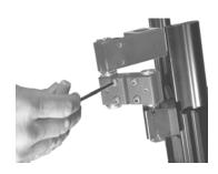
8. Hold the Pitch Mount Shaft so that the black Pitch Pivot is at the proximal end, the hole through the Pitch Pivot is in the line of progression of the chair and the plate of the pivot is facing laterally. Insert the Pitch Mount Shaft into the Mount Shaft Base. Snug but do not tighten the Shaft Screws on the Mount Shaft Base.
