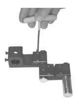
3. Rotate the 3 inch Arm and position the 4 inch Mount Arm onto the Joint Pin as shown. Replace the Arm Clamp and the two Clamp Screws. Tighten the Clamp Screws.
