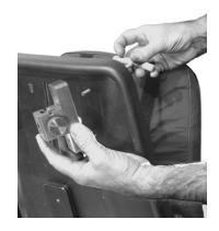
7. Loosen but **do not remove** the Locking Knob on the Mount Base.
