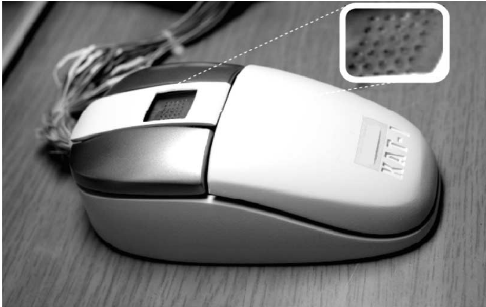
Fig. 20. Prototype of the texture display mouse (Kyung et al., 2007).
