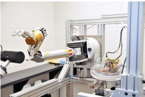
Figure 6. Dexterous kinematic control of a robotic arm and hand by a monkey through a BNCI setup (Credit: Pittsburgh University - Motorlab).
