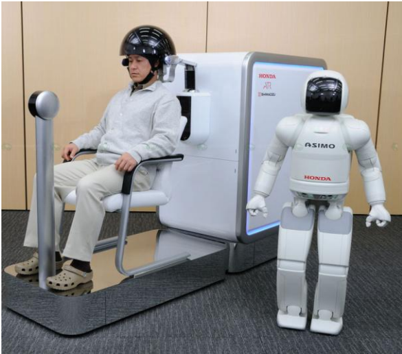
Figure 5. Honda fMRI based BNCI for Asimov robotic platform control (Credit: Honda Research Institute)
