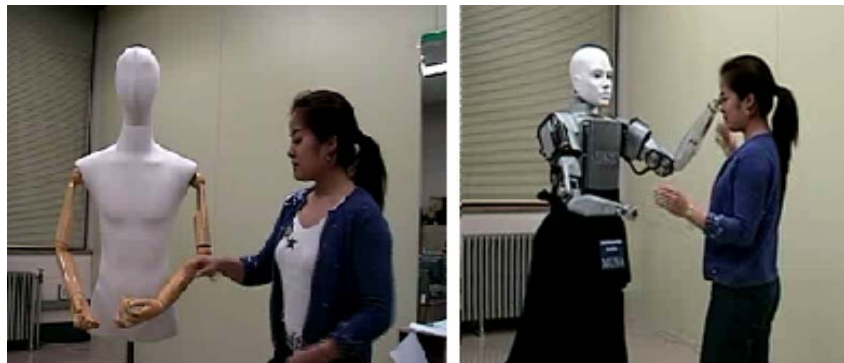
Figure 4.2 Setting up robot arm as if setting up a mannequin on MUSA
