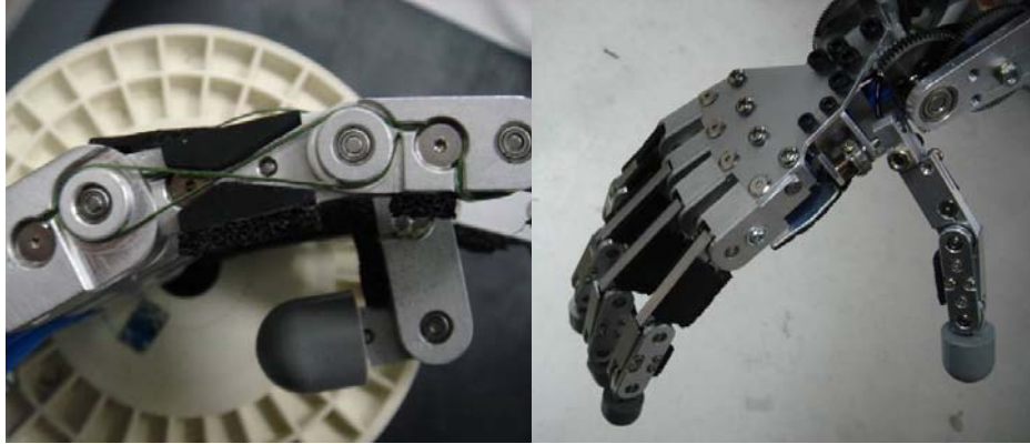
Figure 5.8 Robotic hand's finger joints: machined groove and ball joint thumb
