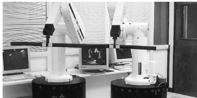
Figure 2.20 Interactive 6-axis F-T sensor installed PUMA arm
