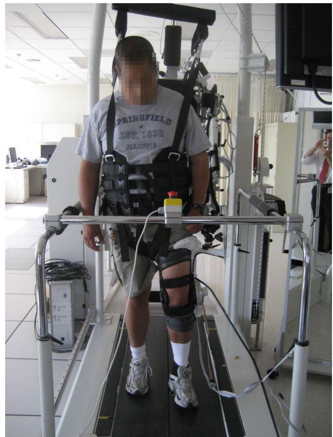
Fig. 5. Experimental setup where a subject wears a harness to be protected from falls. Cables leading to device are for Bowden actuation and sensors, whose weight is partially supported at the bar.
