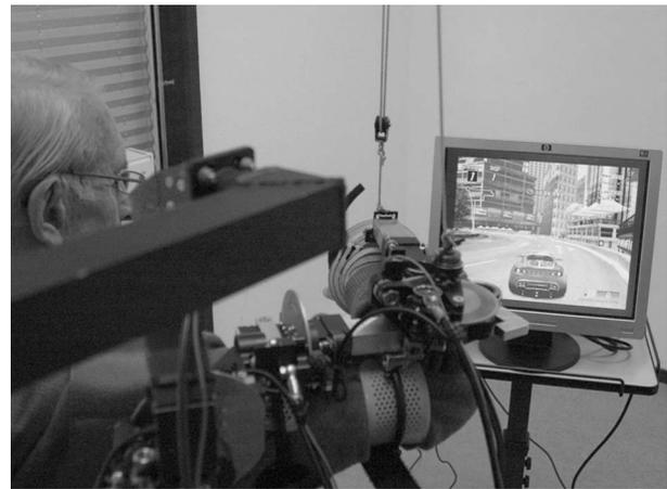
**Fig. 13** Integrated gaming environment connected to the Dampace torques and movements. Either isometric thoracohumeral-elevation torques or isotone rotations are mapped to the gas paddle in the racing game, and either humeroulnar isometric torques or isotone rotations to the steering wheel. Good coordination of simultaneous shoulder and elbow torques is thus required for good driving control in the game and should motivate the subjects to keep exercising.
