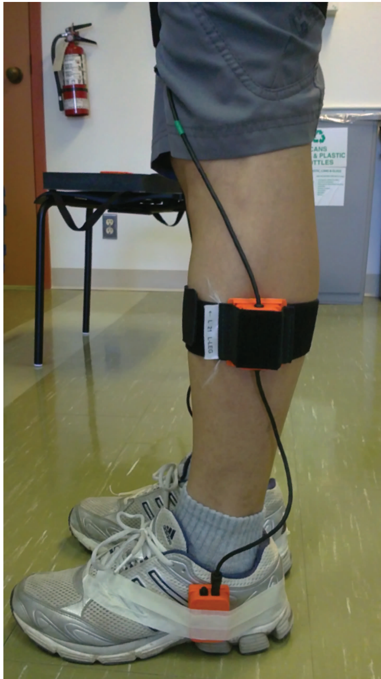
Figure A.1: Shank-mounted IMU based walking speed estimation method sensor configuration.
