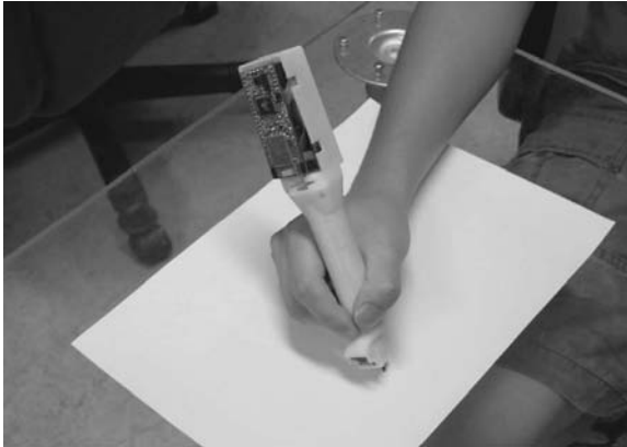
Figure 7.13. Experiment setup for Digital Writing Instrument with MAG- \mu IMU.
