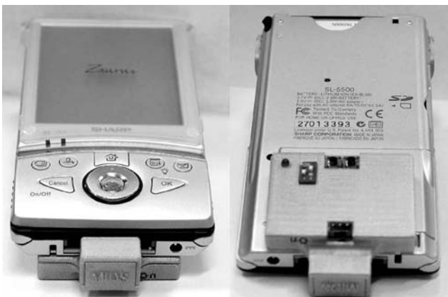
Figure 6.51. Installation of E-MIDS for a Sharp PDA.
