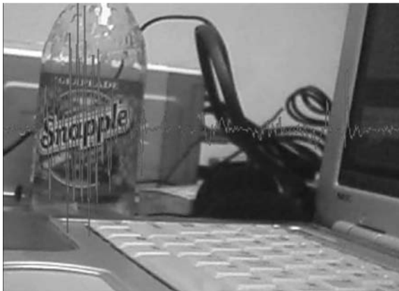
Figure 3.4. Gray-level difference curve of one row in an image.
