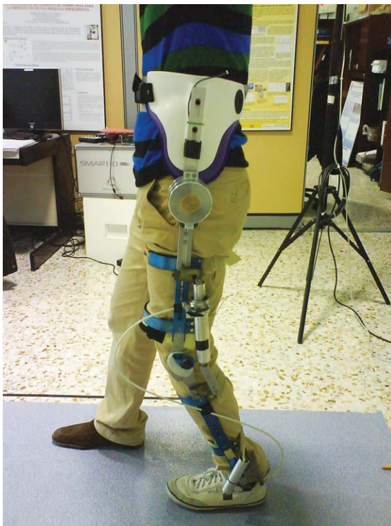
Fig. 10. Lateral view of ESBiRRo HKAFO exoskeleton depicting DC flat motors at the hip, and variable stiffness actuators at knee and ankle.
