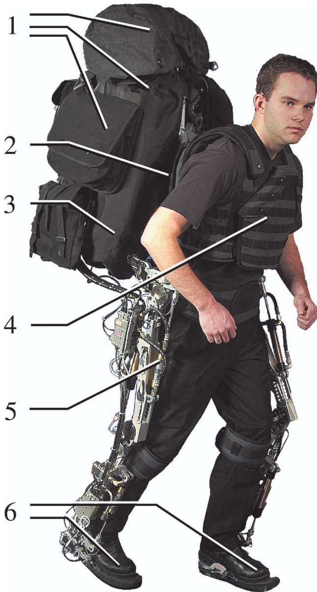
Fig. 1 Berkeley lower extremity exoskeleton (BLEEX) and pilot Ryan Steger. (1) Load occupies the upper portion of the backpack and around the power unit, (2) rigid connection of the BLEEX spine to the pilot's vest, (3) power unit and central computer occupies the lower portion of the backpack, (4) semi-rigid vest connecting BLEEX to the pilot, (5) one of the hydraulic actuators, and (6) rigid connection of the BLEEX feet to the pilot's boots (more photographs can be found at http://bleex.me.berkeley.edu ).
