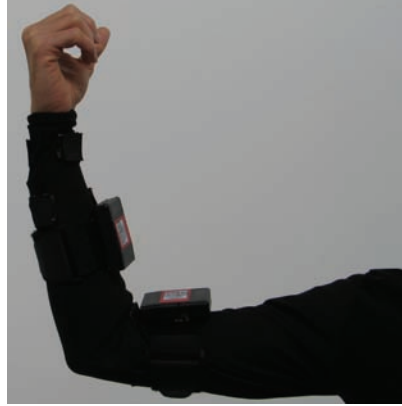
(b) WiTilts mounted on the user's arm.
