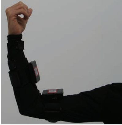
Figure 8.5: WiTilts mounted on the user’s hand to measure the arm’s configuration.
