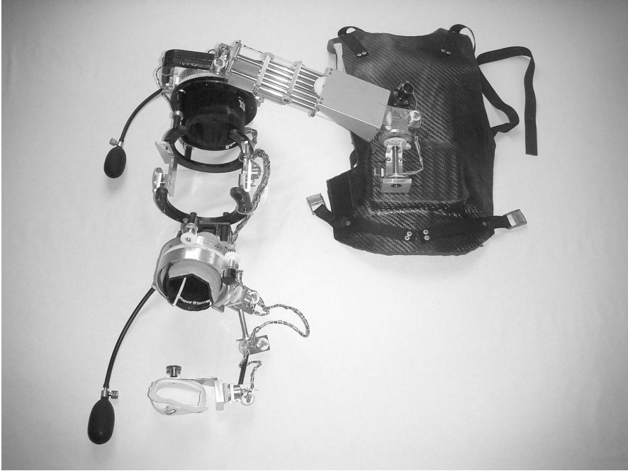
Fig. 3.20. Picture of the ergonomic exoskeleton prototype. The Exoskeleton is attached to a rigid CRP vest and interfaces to the human arm at three levels, the upper arm, forearm and the palm.
