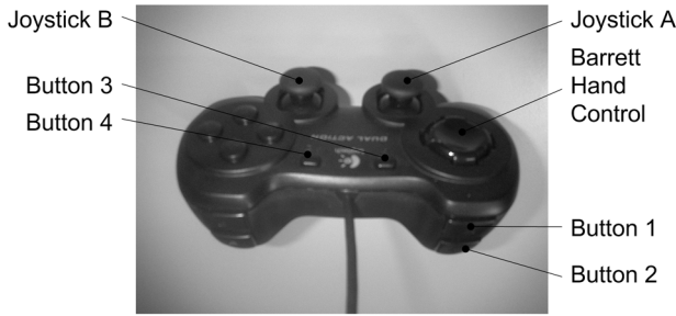
Fig. 7.5. Logitech Dual Action Joystick currently used as input device for robot control experiments. Shown are the buttons that have additional functionality
