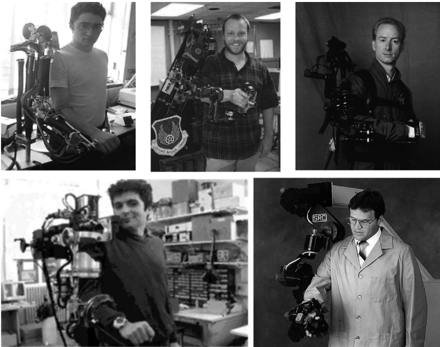
Fig. 1.3. Overview of existing exoskeleton systems. Top (left to right): Salford Exoskeleton, FreFlex Exoskeleton, Exos Inc. Arm Master. Bottom (left to right): Perco Glad-in-Art Exoskeleton, Sarcos Inc. Arm Master
