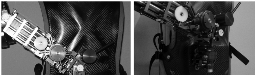
Fig. 13.2. Details of the implementation of drives in the X-ARM-II exoskeleton. The first three joints incorporate the Bowden Cable actuators. Pulleys for the receiving end of the cable transmission can be seen. All pulleys contain torque sensors integrated into their internals.
