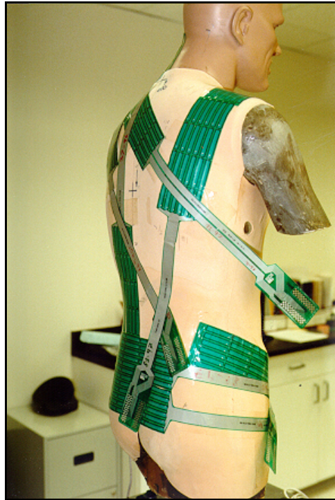
Figure 2. Typical Placement of F-Scan Contact Pressure Measurement System
