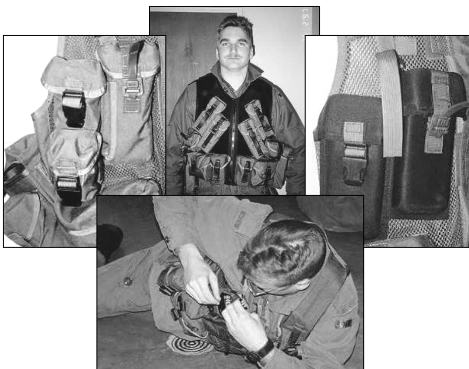
Figure 7. Rapid prototyping vest (top centre) and range of magazine pocket designs and features evaluated for accessibility
