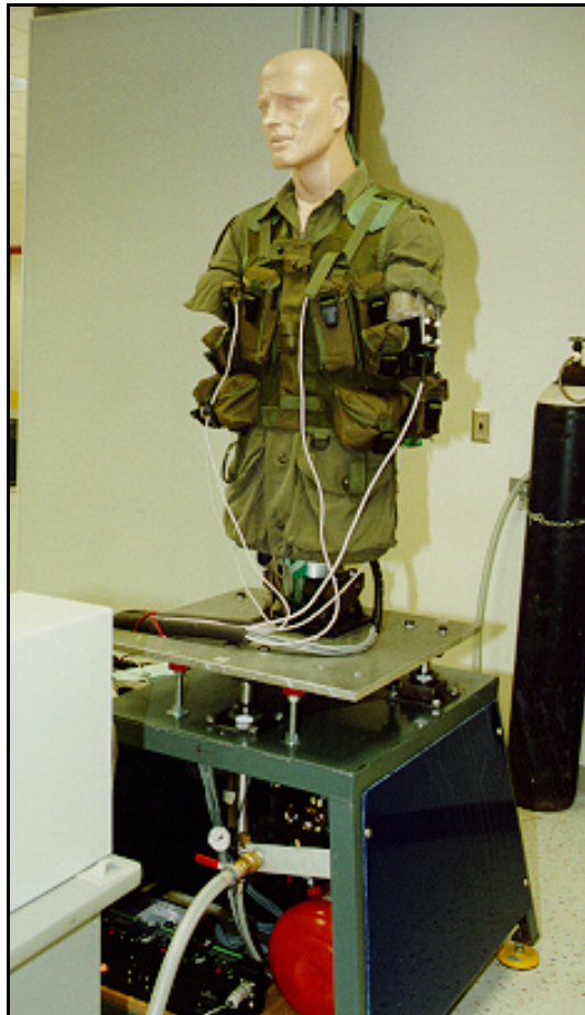
Figure 1. Dynamic Load Carriage Simulator (can be programmed to walk, jog or run and is set-up to test a load-bearing vest design)
