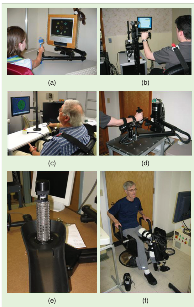
Fig. 2. A gym of robots. (a) The shoulder-and-elbow MIT-MANUS delivering therapy to a child with CP (Spaulding Rehabilitation Hospital). (b) The antigravity module (Baltimore VAMC). (c) A person with PD and deep brain stimulation (DBS) practicing with the wrist robot (University of California San Diego). (d) The integrated system affording whole-arm training (transport of the arm and manipulation of objects, VA Coop Study Randomized Clinical Trial CSP 558). (e) The hand module (without cover). (f) A person with MS during therapy with the anklebot (West Haven VA Medical Center).
