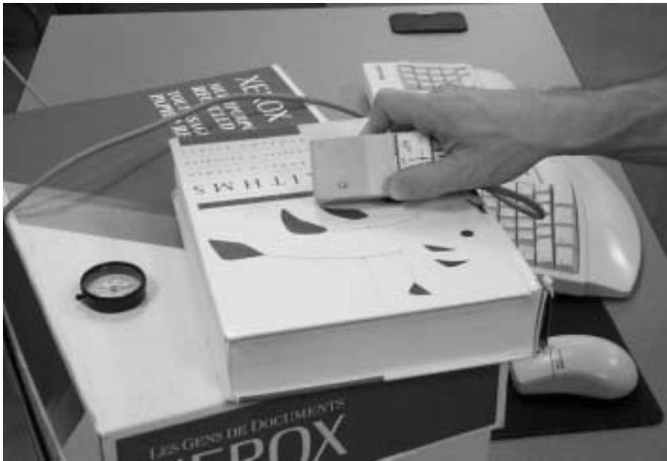
Figure 23: Rotating Sensor 90 Degrees About Positive x -axis For Rate Calibration
