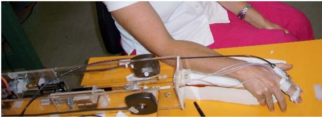
Figure 7.7 The position and orientation of subjects in respect to the platform. A non-injured subject is shown with her finger in the experimental harness.
