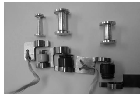
Figure 7: Components of the exoskeleton finger. Three torsion springs hold each section together. They are supported by inner sleeves (shown above springs) and are encased by plastic bearing sleeves
