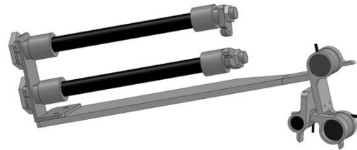
Figure 6: CAD model of prototype two showing three torsion springs and two PMAs used as the actuators. Bowden cables and sensors are not depicted.
