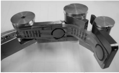
Figure 9: Placement of the two dorsal side force sensors which sit along the back of the finger.
