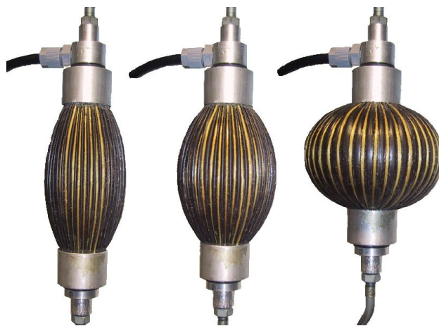
Fig. 1. Pleated pneumatic artificial muscle at different contraction levels
