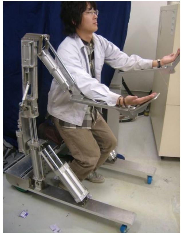
Fig. 1 : Position of the caretaker in the slave system. Note that oil tubes and caretaker's arm's protective parts are missing in this picture.
