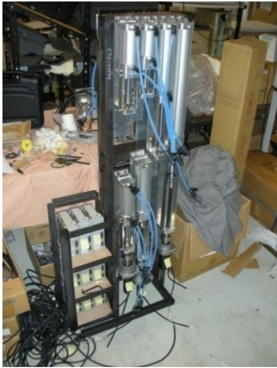
Fig. 2 : Master unit. Note : the oil pipes between the master and the slave unit are missing, and this pictures only shows cylinders of only one side of the unit.
