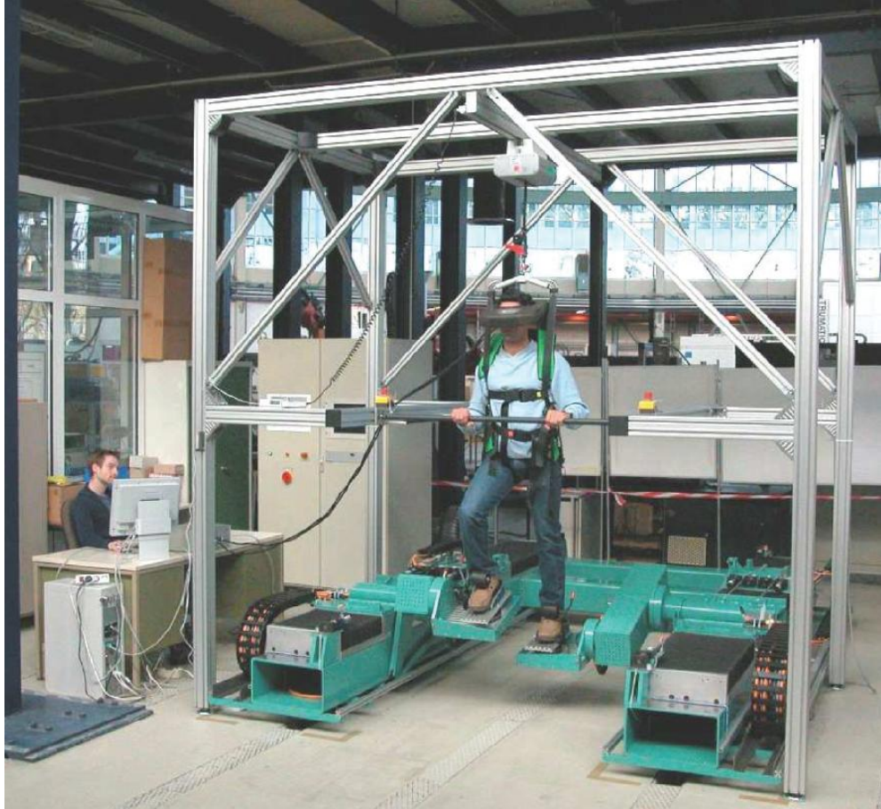
Figure 7. Robotic walking simulator: HapticWalker, [Schmidt et. al., 2005].
