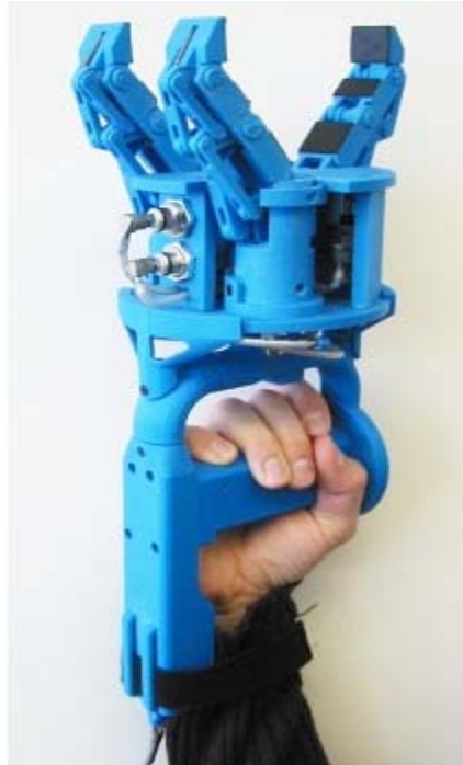
Figure 8: The pneumatic model is much smaller than either of the previously created models, although a compressor is needed to provide air pressure.
