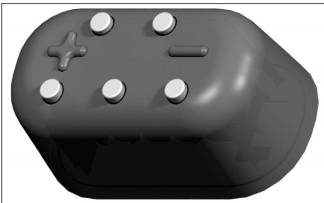
Figure 10. Control unit with five switches to adjust balancer settings of arm support.
