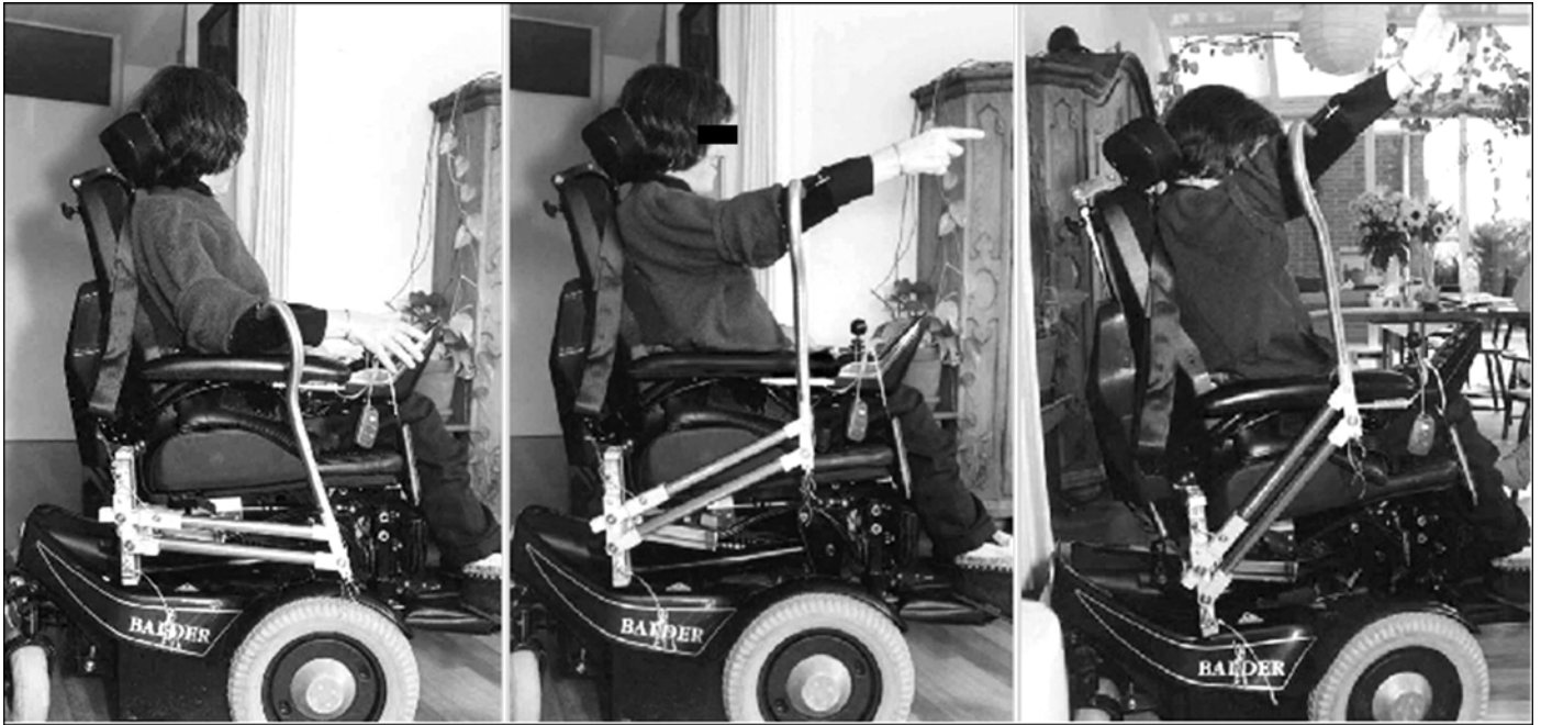
Figure 3. User (spinal muscular atrophy patient) demonstrating her increased range of motion with first arm support prototype.
