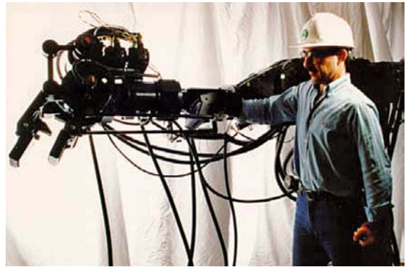
Fig. 33.4 One-handed upper-extremity exoskeleton where a gripper allows for grasping of heavy objects [33.21]
