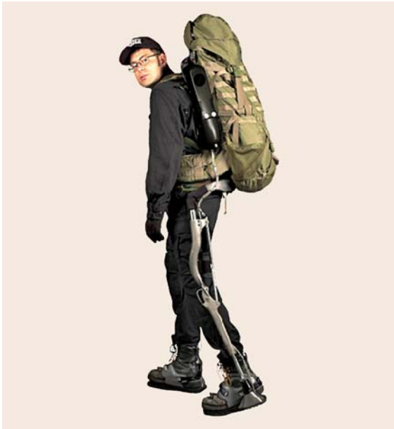
Fig. 33.28 The ExoClimber™ field-ready exoskeleton is suitable for rapid ascent of stairs and steep slopes (courtesy of Berkeley Bionics, Oct 2005)
