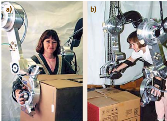
Fig. 33.3a,b Two-handed upper-extremity exoskeleton where artificially built friction forces between the load and the arms allow for grasping objects [33.25]
