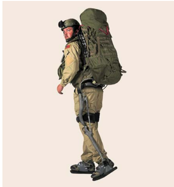
Fig. 33.25 The ExoHiker™ field-ready exoskeleton is suitable for small slopes and can carry a load of 90 kg (courtesy of Berkeley Bionics, Jan 2005)
