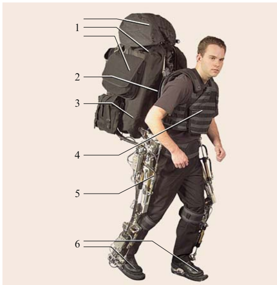
Fig. 33.10 Berkeley lower-extremity exoskeleton (BLEEX) and pilot Ryan Steger. 1: The load occupies the upper portion of the backpack and around the power unit; 2: rigid connection of the BLEEX spine to the pilot's vest; 3: the power unit and central computer occupies the lower portion of the backpack; 4: semirigid vest connecting BLEEX to the pilot; 5: one of the hydraulic actuators; 6: rigid connection of the BLEEX feet to the pilot's boots
