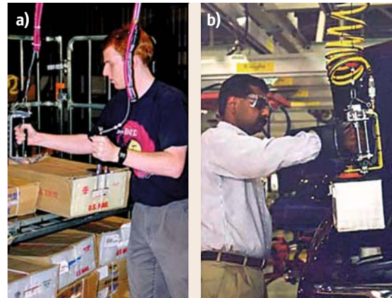
Fig. 33.9a,b The use of IADs for mail and package delivery service (a) and automobile industries (b)
