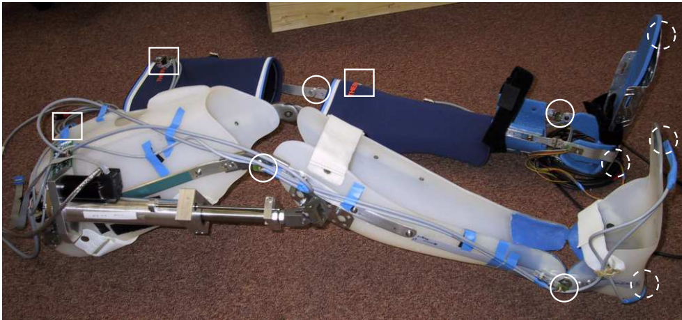
Figure 8.4: Early stage of the actuated orthosis (foreground). The leg brace used to hold the sensors for measuring the joint angle information from the unactuated leg is shown in the background. Squares indicate the position of the accelerometers, circles mark Hall sensors, and dashed circles show the location of the floor contact sensors.
