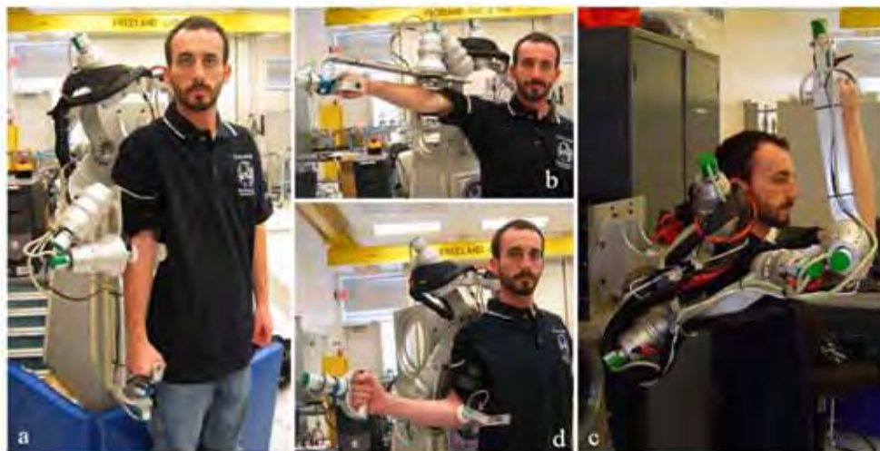
Fig. 4. Exoskeleton shown at (a) full shoulder adduction (b) 90 degree shoulder abduction, (c) mid-elbow flexion, and (d) near full lateral rotation.
