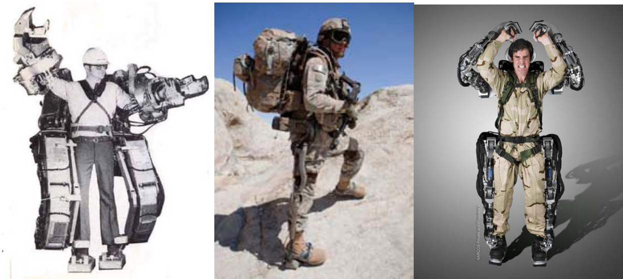
Figure 7 The Figure shows the evolution of military exoskeleton technology. From left to right: 1963 General Electric/Office of Naval Research HARDIMAN project, The Berkely Bionics/Locheed Martin HULC, and the SARCOS Labs/Raytheon XOS. HULC is a lower body exo design to support roughly a 10:1 ratio carrying capacity, is battery powered, and performs assisted walking and load transfer through the skeleton to the ground. XOS is a full body design for strength augmentation that currently supports roughly a 25:1 ratio and is powered from a tethered source. HULC supports an infantry-type mission and XOS is envisioned for rear area support for such tasks as heavy lifting, powered tools, and repetitive load tasks. (Source: Dollar and Herr article, HULC product card, U.S. Army Natick Labs)
