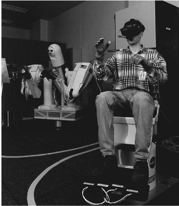
Fig. 5. NASA JSC full immersion telepresence testbed (after [6]).
