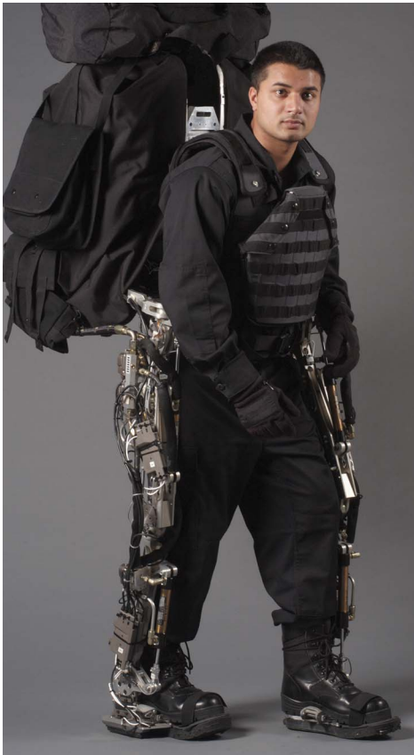
Fig. 16 Final BLEEX Design
