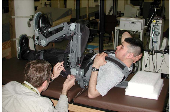
Fig. 5 BLEEX Mock-up used to test and revise the BLEEX degrees of freedom, ranges of motion, and ergonomics. These prototypes were built on a Fused Deposition Modeling (FDM) machine.
