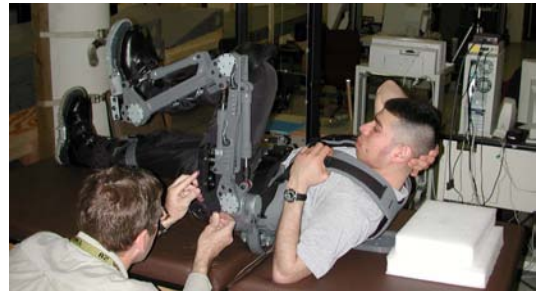
Fig. 14. One of the functional mock-ups of the exoskeleton architecture created at UC Berkeley to determine necessary degrees of freedom, ranges of motion, and ergonomic attachments. These prototypes were made by a Fused Deposition Modeling (FDM) machine.
