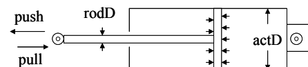
Fig. 15. Bi-directional linear hydraulic actuator schematic. Note that the area on which the internal pressure can act is different on the piston and rod sides of the actuator. This means that the actuator can push with more force than it can pull given the same supply pressure.
