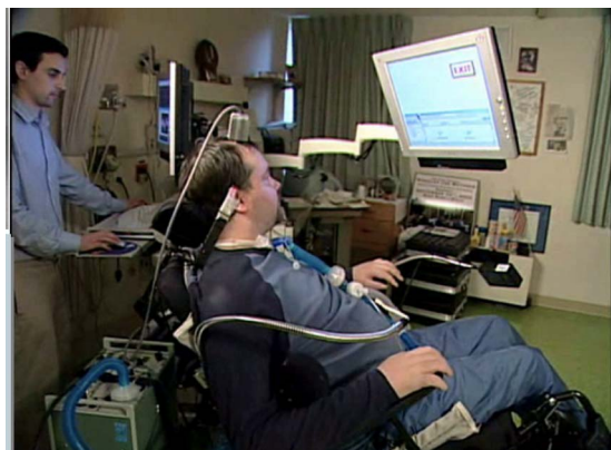
Fig. 3. Photo of a subject patient in a human clinical pilot trial, operating a cursor on a display screen by direct cortical “thought-to-action” control (after [24], [62] and courtesy of BrainGate2.org). The implanted multielectrode array is connected via a skin penetrating wirebundle to a head-mounted stage for analog signal amplification. This stage is tethered to other signal processing (digital) and neural signal decoding electronics in the subject’s vicinity, and the operation is supervised by trained technical personnel.
