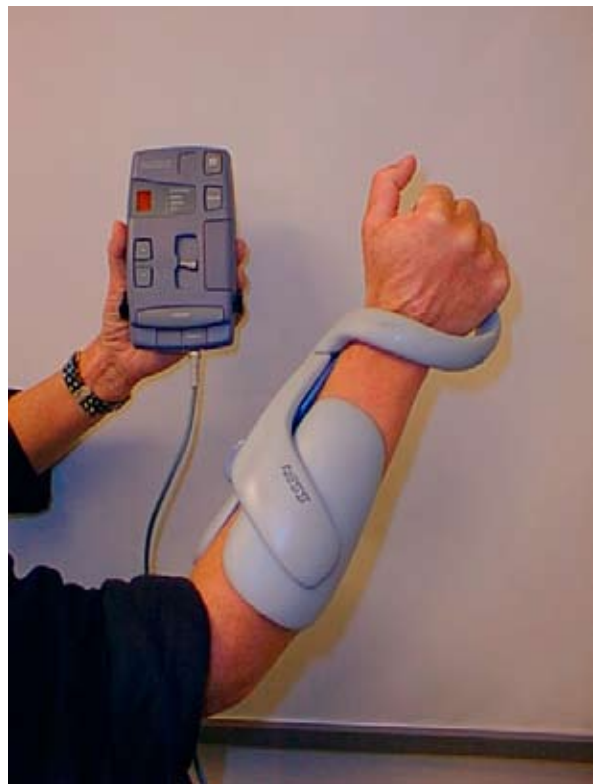
Figure 1. A hybrid brace-transcutaneous neuroprosthesis system (NESS H200) that is worn on the hand and forearm. The exoskeleton positions the wrist in a functional position and the five surface electrodes built into the exoskeleton stimulate specific muscles to provide coordinated hand opening and closing. (Courtesy of Bioness Inc., Santa Clarita, CA)
