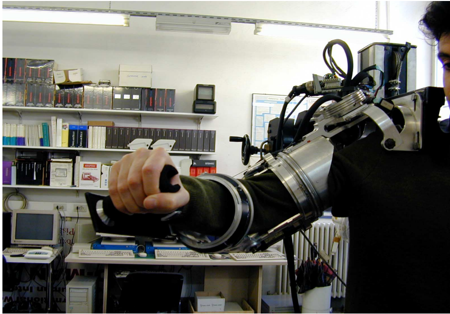
Figure 2 The arm force feedback exoskeleton
