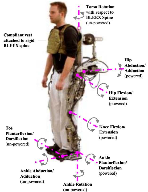
Fig. 2. BLEEX mechanical structure and degrees of freedom.
