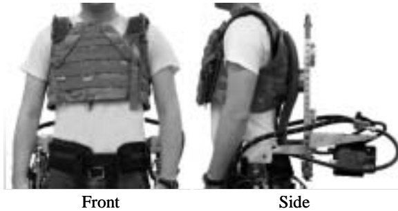
Fig. 3. The pilot vests in this figure and in Figure 1 are designed to uniformly distribute the BLEEX-pilot force on the pilot's upper body (note that the BLEEX power supply is not attached in the "side" image).
