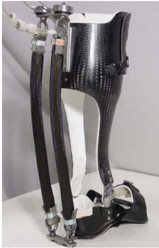
Fig. 1. Subjects wore a custom-made exoskeleton on their left lower limb. The exoskeleton consisted of a carbon fiber shank section and a polypropylene foot section. The exoskeleton was hinged at the ankle to allow free sagittal plane rotation. The exoskeleton had an average weight of 1.08 \pm 0.09 kg (mean \pm SD) and moment arm length of 11.0 \pm 1.2 cm that varied and depended on the size of the subject. Electrical signals (EMG) of soleus were recorded and processed to be used to control air pressure in the artificial pneumatic muscles proportionally. As air pressure increased, the artificial muscles started to develop tension and become shortened, allowing the powered exoskeleton to provide plantar flexor torque controlled by soleus muscle activation.
