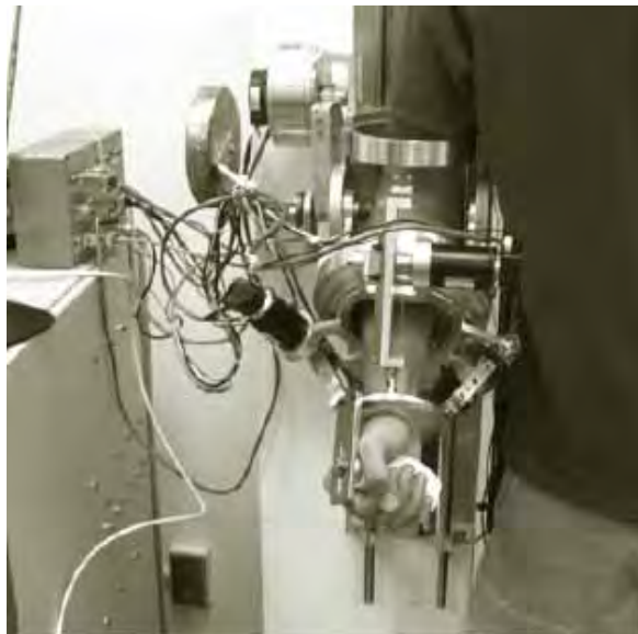
Fig. 5. User operating the MAHI arm exoskeleton.
