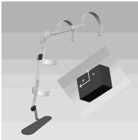
Fig. 23. Configuration of the IMUs in the structure.
