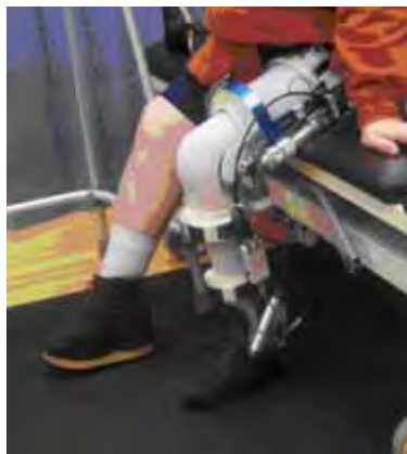
Fig. 26. Image of the wearable exoskeleton on a patient after fitting to the anatomy.
