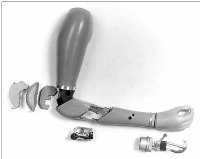
The original Utah Artificial Arm was developed in 1980. The internal control circuits are housed in smooth molded plastic covers that are light, strong, and cosmetic.
