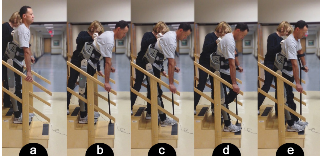
Fig. 5-3. Stair descent sequence, showing a) starting posture, b) leaning forward for CoP trigger, c) extension of right leg over subsequent stair tread, d) lowering of body and right foot to subsequent stair tread, and e) movement of left foot to subsequent stair tread.
