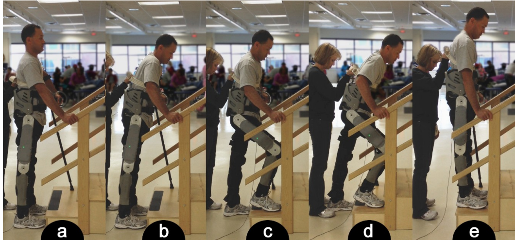
Fig. 5-2. Stair ascent sequence, including a) starting posture, b) leaning forward for initial CoP trigger, c) lifting of right leg to subsequent stair tread, d) leaning forward for second CoP trigger, and e) lifting of body and placement of left foot on subsequent stair tread, next to right foot.
