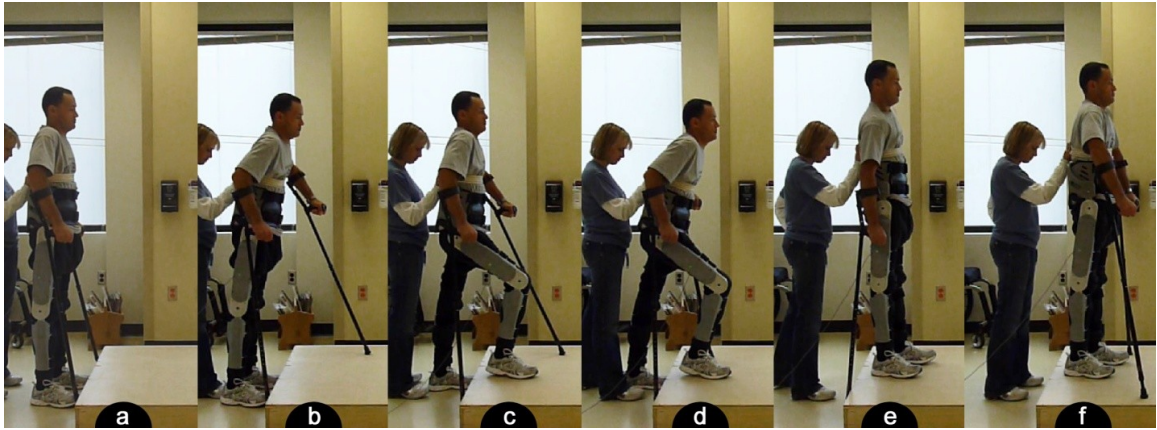
Fig. 5-10. Curb ascent sequence. (a) Starting posture, (b) Leaning forward for CoP trigger, (c) First motion completed, (d) Leaning forward for CoP trigger, (e) Second motion completed, (f) Weight shifted forward with crutches.
