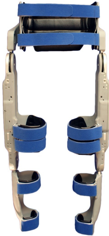
Figure 2-2. Vanderbilt gait restoration orthosis frontal view.
