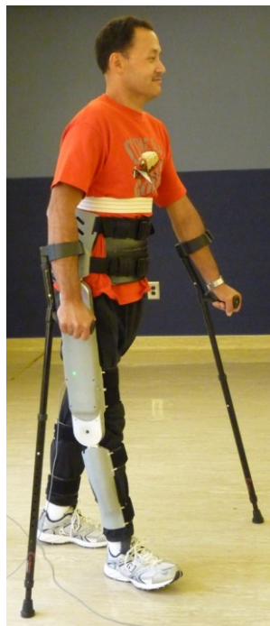
Figure 4-3. T10 complete paraplegic subject wearing Vanderbilt exoskeleton.
