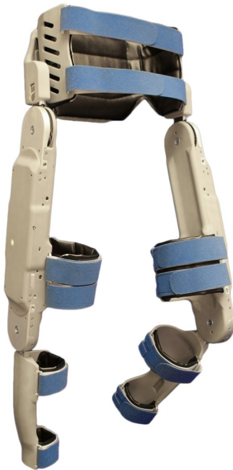
Figure 2-1. Vanderbilt gait restoration orthosis oblique view.
