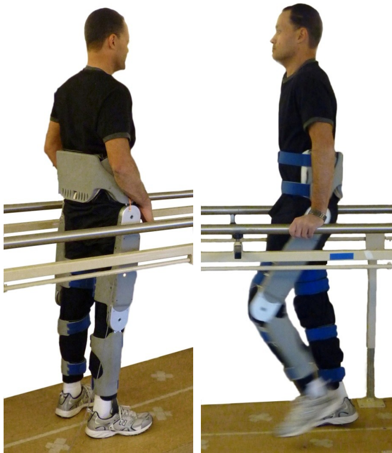
Figure 2-6. Subject with T10 complete spinal cord injury walking wearing the powered orthosis.
