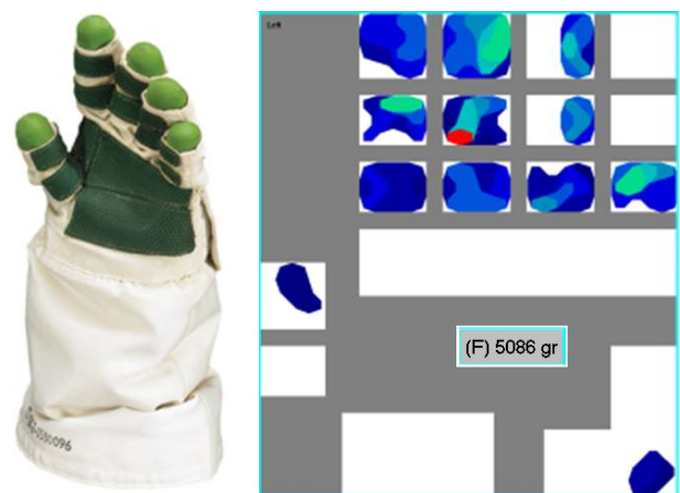
Figure 4. Orlan EVA glove (left) and its effect on the sphere grip test (right)
