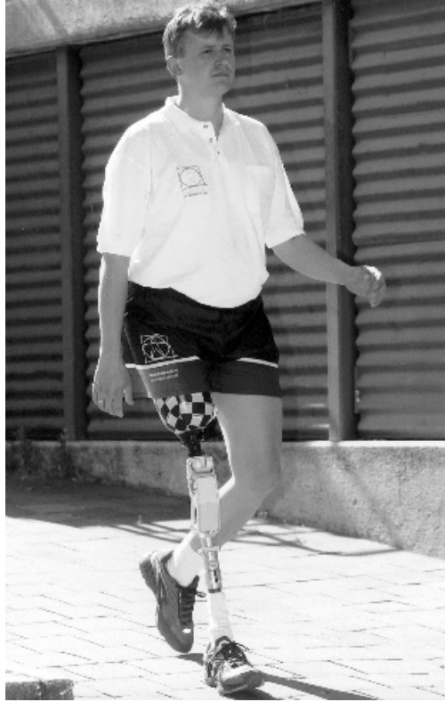
Figure 6.16 A Prolite™ Smart Magnetix™ Above-the-Knee (AK) Prosthesis user walking down a slope: the characteristics required for the knee prosthesis will generally be different from other walking conditions. The MR technology provides the desired adaptation (Reproduced by permission of Lord Corporation).
