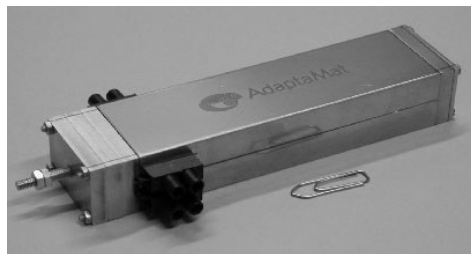
Figure 5.16 A5–2 MSMA actuator prototype from Adaptamat Ltd. (Photograph courtesy of E. Pagounis, Adaptamat Ltd.)
