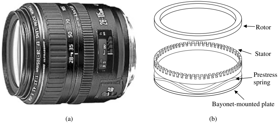
Figure 2.37 Canon lens including a travelling wave ultrasonic motor: (a) view of the lens and (b) schematic view of the 62-mm M-1 USM.
