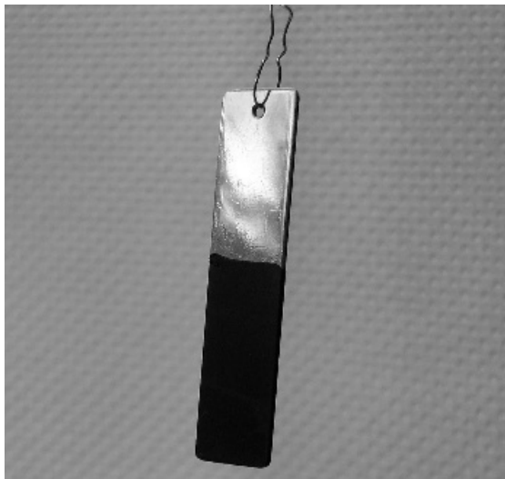
Figure 4.4 A 20- \mu\text{m} polypyrrole (PPy) actuator electrochemically grown on a 1-cm stainless steel electrode. Courtesy of S. Skaarup, DTU.
