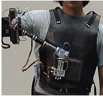
Figure 8: Shoulder assembly attached to human operator (left: Exoskeleton Prototype, right: Artist impression)
