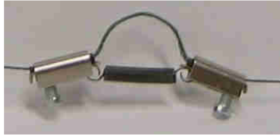
Figure 5.9: Artificial tendon spring-slack arrangement emulating the natural tendon's compliance
